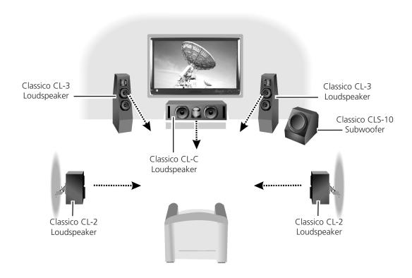
Figure 4. Example of a Surround Sound (5.1 Configuration) Setup
