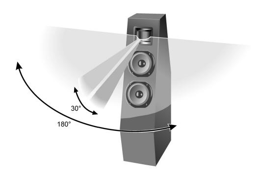
Figure 1. Dispersion Pattern of the CDT<sub>3</sub> Tweeter
