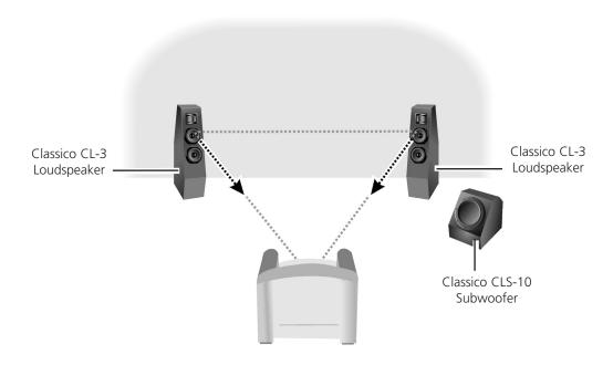
Figure 3. Example of a Stereo with Subwoofer (2.1 Configuration) Setup
